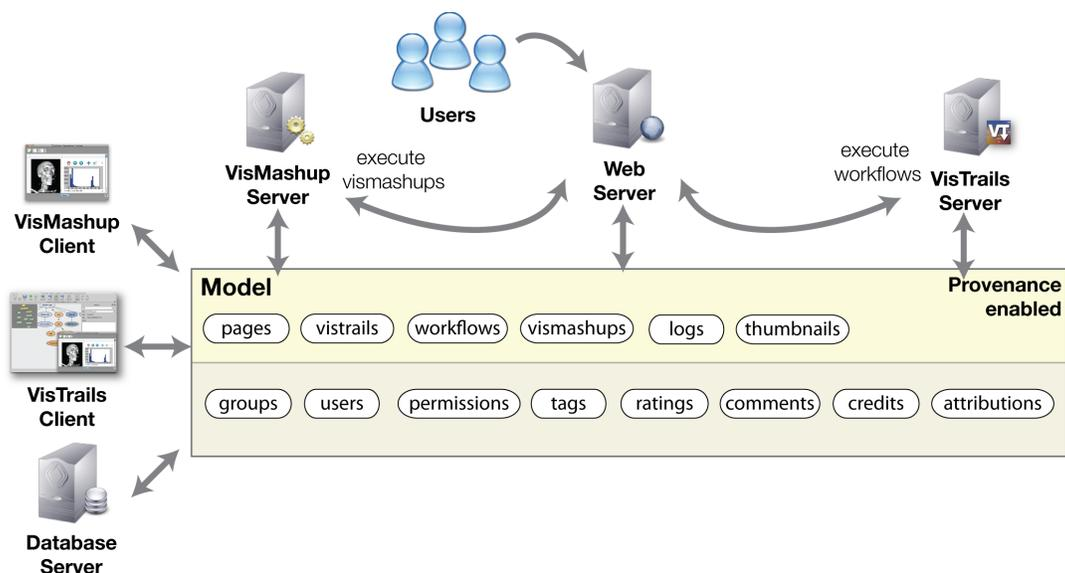
Figure 1. Architecture of the social data analysis site based on VisTrails and VisMashup. The VisTrails provenance model is shared with all the other other servers and client applications in the architecture. The data model is also extended to include the social Web features such as groups, permissions, ratings and comments. Mashups and workflows embedded in web pages are executed in the servers and the results are displayed in the web page.
